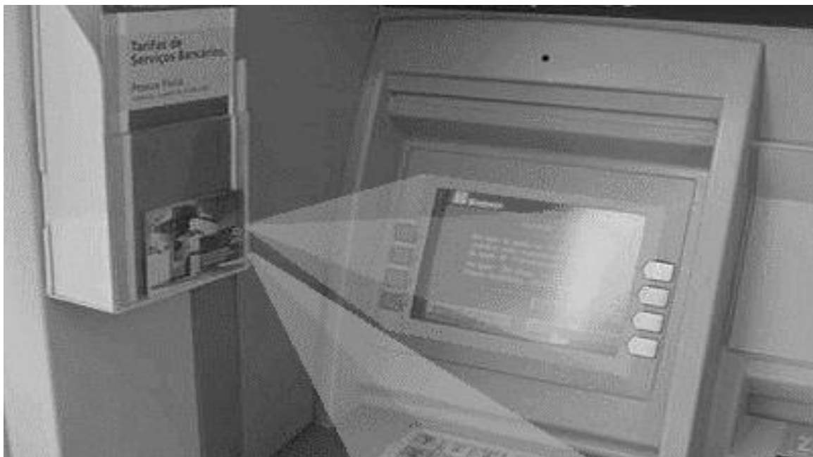
The micro camera mounted in the side of the fake pamphlet box can view the KEYPAD and MONITOR, and transmits wireless pictures up to 650 feet away.
